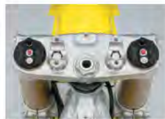
*Prednja vilica PSF2 (pneumatski amortizer KYB)
